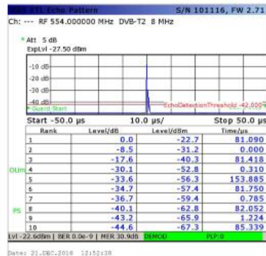
Figure 6. The levels and time lags of the signals at the output of the Gap Filler, connected to the artificial antenna
