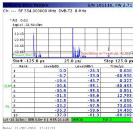
Figure 11. The levels and time lags of the signals transmitted by the Gap Filler (Pout = 50 W), TVA 31/50 broadcast antenna, \Delta\phi = 110 gr.
