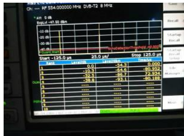
Figure 4. Measurement of input signal levels and their arrival time
