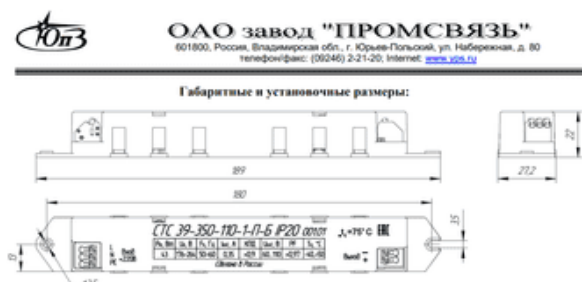
Figure 7. Power block CTC 39-350-110-1-П-Б IP20 001.01
