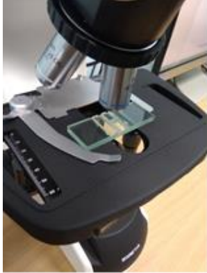
Fig. 4 - Microscope with Goryaev's camera located on the subject table
