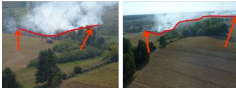
Figure 3. Estimated fire front after arriving to the fire scene without drone supported reconnaissance (left) and with drone supported reconnaissance (right). Source: author
